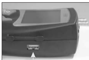
USB port for connection to the printer and joining to a PC
